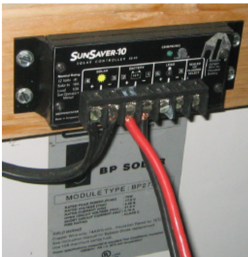
75 watt solar panel with controller mounted on the back of the panel
