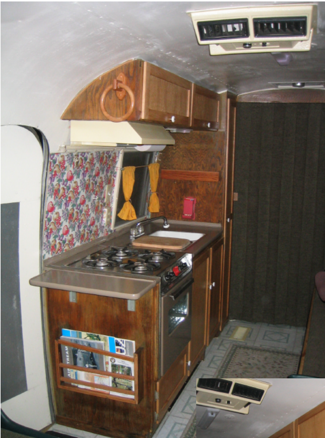
Galley w/ original Magic Chef stove/oven. Original furnace is located beneath the right side of the sink with two registers and a duct to the black water tank to keep it from freezing. I would like to upgrade to a digital thermostat.
