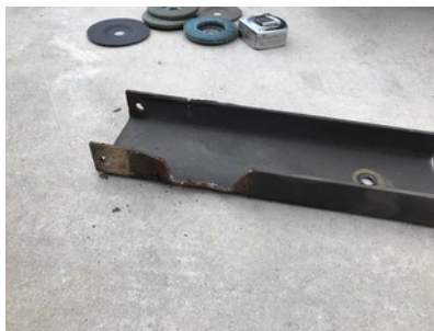
This is the other side of the hitch mounting rail. The bent parts were cut out and two pieces of 3" x 1/4" flat steel were going to be welded both on top and on bottom of the length of the mounting rail to provide a heavier, and much added support of the hitch receiver.
