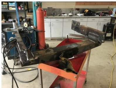
Angle gussets were also added to provide more support of the hitch receiver. The goal was to over build the hitch so I would never again have to go through this experience!!
