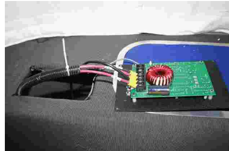
4: Wiring Harness at MPPT Charge Controller
