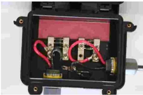
3: Street Side Junction Box & Series Wiring
